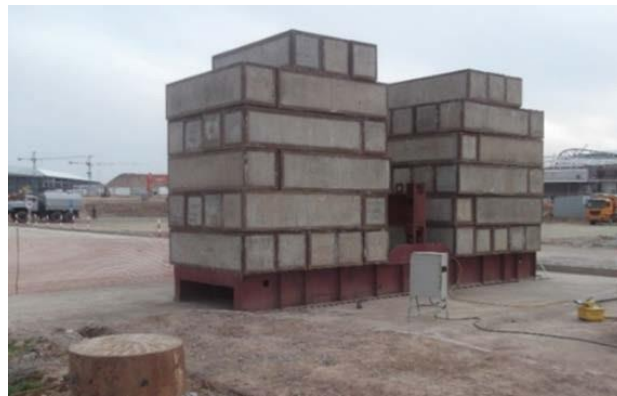
Fig. 2. Static load test on construction site.
